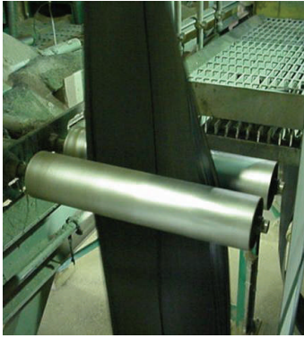
CRODON pipe used to move roofing shingle mat.
