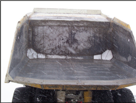
CRODON Punched Plate Screen Improves Flow and Improves Life
