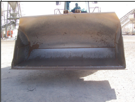
CRODON In Loader Buckets Extends Life and Prevents Carry-Back
